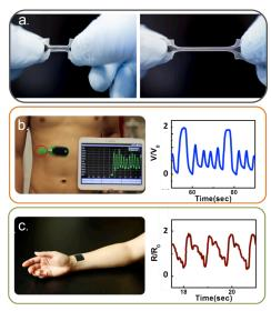
**Figure 1:** Physiological monitoring with conformal sensors. (a) Shows how soft and stretchy the piezoresistive sensors are. (b) Respiration monitoring (including tidal volume) and (c) radial artery pulse waveform.
